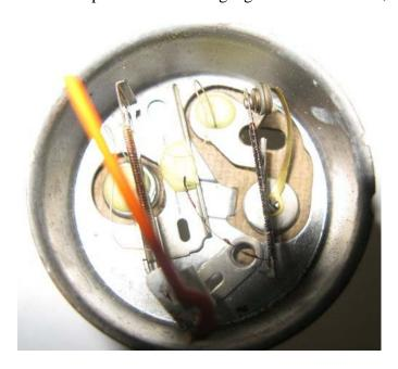
Step 2: Bend the limiter points out of the way, so that they no longer contact. Make sure that the points don't touch anything.
