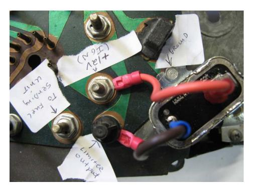
• Step 7: Test the setup by turning the key on in the car. The fuel gauge, oil gauge, and temperature gauge should operate properly, and the red LED on the new solid state limiter should blink after the 3-6 second warm up time.
